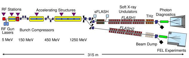
Figure 1: The FLASH facility with the injector, the main linac, and the two beam lines FLASH1 and FLASH2. (Not to scale.)
