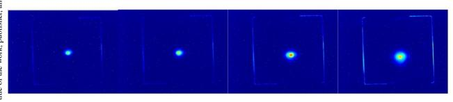
Figure 2: FLASH2: FEL beam spot on Ce-YAG screen for various wavelengths obtained by changing the undulator gap within about 30 min. for all wavelengths. From left to right: 6.0 nm, 8.5 nm, 11.0 nm, 13.5 nm.
