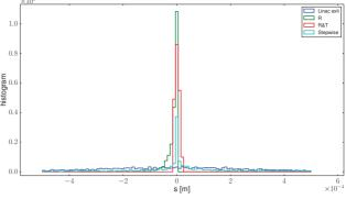
Figure 6: Histograms of the longitudinal bunch distributions of Figure 5. While a compression of the very center of the bunch is possible, long tails are found.
