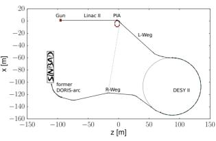
Figure 1: The geometric layout of the beam transport system from the electron gun of Linac II up to the SINBAD facility.
