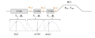
Figure 1: Layout of an x-band FEL accelerator design, up to end of first bunch compressor, which employs Phase Modulation Linearization. Included are markers showing location of longitudinal phase space plots in Fig. 3.
