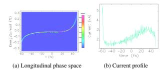
Figure 7: Beam properties at the end of Linac2, utilizing Harmonic Linearization.
