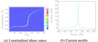
Figure 5: Beam properties at the end of Linac2, utilizing Phase Modulation Linearization.
