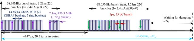
a) Detailed time structure in mid-cycle 1, fills the 1st of every 7 buckets
