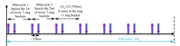
b) Time structure of a full injection cycle, fills every bucket of the two bunch trains in the ring one time Figure 5: Injection cycles (not to scale)
