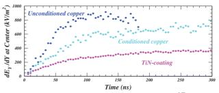
Figure 6: Electron cloud vertical field gradient  $\frac{dE_Y}{dY}$  on the beam axis versus cloud buildup time.
