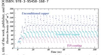
author(s), Figure 4: Beam-pipe-averaged cloud densities in the absence of the quadrupole and solenoidal magnetic fields.
