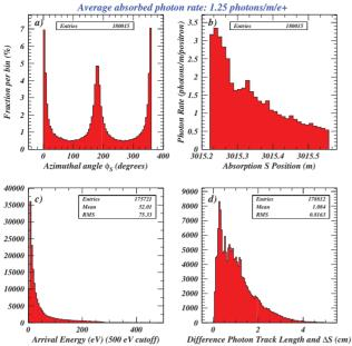
Figure 2: Distributions of photons absorbed in the finalfocus quadrupole magnet QC1RP including the effects of photon scattering in the positron ring. a) Distribution in azimuthal angle  $\phi_s$  of the absorbed photon position around the 21-mm-diameter beam pipe. b) Distribution of absorbed photon locations in the arc coordinate S of the positron orbit. c) Distribution of absorbed photon energies below 500 eV. d) Difference of photon and positron orbit track lengths.
