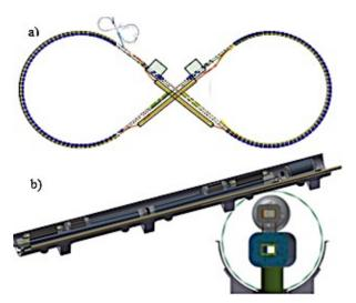
Figure 1: a) MEIC Ion Ring configuration, showing an overlay of an ECR with its cooling straight sections displaced; b) half-cell cryostat of the Ion Ring lattice, showing a full-cell of the ECR mounted piggy-back.
