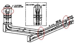
Figure 3. Schematic view of electron beam for ECR (from [7]). Red regions highlight the transitions between immersed Brillouin flow and periodically lensed flow of the electron beam.
