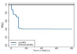
Figure 6: Normalised number of circulating particles for  $8 \cdot 10^4$  turns in the LHC, with (blue) and without (black) a HEL operating in Diffusive mode.
