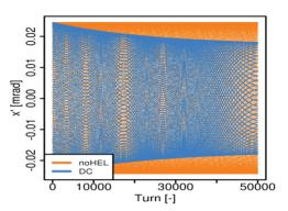
Figure 2: Particle motion in the LHC driven by a DC HEL (blue), compared to no HEL (orange), at the primary collimator ( $s \approx 19790m$ ).
