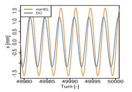
Figure 3: Particle transverse *x* position at the primary collimator ( $s \approx 19790m$ ) in the LHC after 49980 turns. Position with (blue) and without (orange) a DC HEL has been fitted with a sinusoid to illustrate a tune shift of order  $\approx +3 \cdot 10^{-4}$ .
