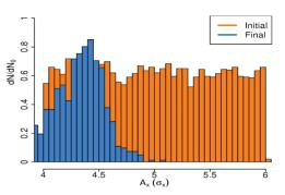
Figure 5: Normalised inital (blue) and final (orange) particle distributions for  $8 \cdot 10^4$  turns in the LHC with a HEL operating in Diffusive mode.
