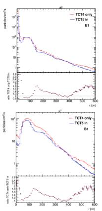
Figure 5: Transversal radial distributions for all particles (top) and muons (bottom) at the interface plane.
