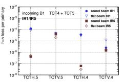
Figure 3: Comparison of losses on TCTs for round ( $\beta_{x,y}^*$  is 15 cm) and flat ( $\beta_{x/y}^* = 7.5$  cm,  $\beta_{y/x}^* = 30$  cm) beam optics.
