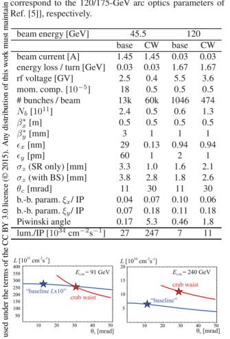
Figure 1: Luminosity per IP vs. full crossing angle. The stars indicate the operation points of Table 1.
