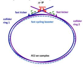
Figure 1: Schematic γγ collider based on filling the two FCC-ee collider rings with  $e^{-}$  bunches and extracting one bunch per beam and per turn into a dedicated  $\gamma\gamma$  line.
