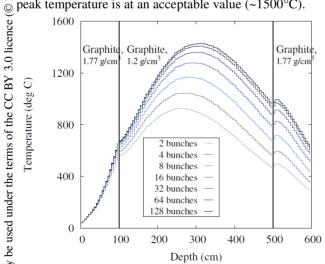
Figure 2: Longitudinal peak temperature profile induced by 50 TeV proton bunches  $(1 \times 10^{11})$  in a LHC-like dump core. Bunches are assumed to have a size of 400 µm this  $(=1\sigma)$  and a transverse separation of 1.6 mm.
