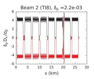
Figure 2: Worst-case off-momentum trajectory in the LHC for beam 2 with a momentum cut of  $\Delta p/p = \pm 0.22\%$  in TI 8.
