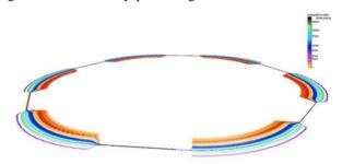
Figure 8: Electron beam trajectories for both NS-FFAGs around the whole RHIC tunnel (without by-passes) magnified transversely 5000×.
