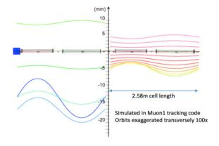
Figure 2: Electron orbits in the eRHIC arc cells, magnified 1000x transversely: lower energy loop 1.3-6.6 GeV (left); and high-energy loop 7.9-21.2 GeV (right).
