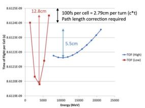
Figure 4: Time of flight dependence of the two eRHIC
