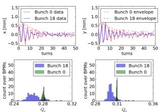
Figure 3: Raw data from one LHC BPM of bunch-by-bunch H/V injection oscillations for 2 bunches (top) and distribution of tune estimates from all BPMs. Bunch 0 is the first of the injected train, while 18 is in the middle of the PS batch. The raw data and the envelope (from a Hilbert transform), show the difference in damping times, which is reflected in the accuracy of the corresponding tune estimates.
