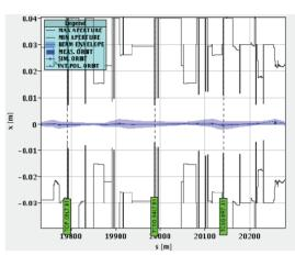
Figure 1: The IR7 horizontal aperture and beam orbit, with the envelope denoting the  $1-\sigma$  beam size. The green text boxes show names of a few IR7 horizontal collimators.
