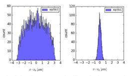
Figure 2: Orbit deviation at the IP in the horizontal plane for Beam 1 if the the crossing scheme is matched without weights (left) and with increased weights of the constraints representing the BPMs between D1L and D1R (right).
