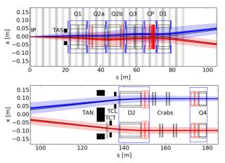
Figure 1: Sketch of the Layout on the Right Side of IP1 and IP5 from the IP to D1 (top) and from D1 to Q4 (bottom). Dark blue and red area show the  $2\sigma$  beam envelops of Beam 1 and Beam 2. Light blue and red areas show the 12  $\sigma$ beam envelops with imperfections (20% beta beating and 2 mm orbit error). On the top plot, gray bands highlight the location of the parasitic encounters for 25 ns bunch spacing and small blue boxes the BPMs.
