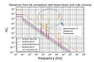
Figure 2: Tolerances from DA simulations expressed in terms of horizontal tune shift. A similar plot is obtained for the vertical plane. The red line of the Baseline powering scheme is superimposed over the pink line for the Q1Q2a-Q2bQ3 powering scheme.
