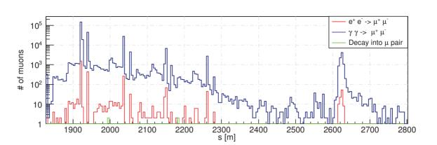
Figure 4: Origin of muons along the BDS from primary electrons hitting to the first spoiler in betatron collimation section.
