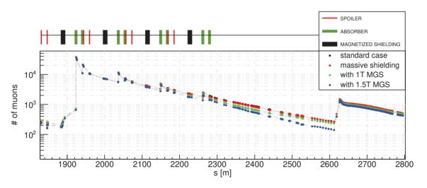
Figure 5: Effect of magnetized shieldings to the muon flux in betatron collimation section.
