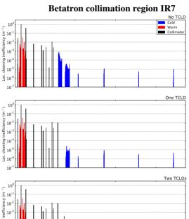
Figure 2: Simulated loss maps with and without the TCLD collimators for the full LHC ring and the betatron collimation region IR7.
