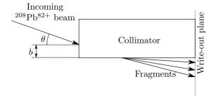
Figure 1: Schematical illustration of the fragmentation simulation. The collimator is modeled as a block of carbon. A beam of  $^{208}\text{Pb}^{82+}$  ions hits the material at an angle  $\theta$  with an impact parameter b. At the end of the collimator, the coordinates and species of all ions are written out.
