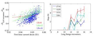
Figure 7: Left: Correlations between the long-range beambeam observable with the first hour current decay and the number of long range encounters for fill 3232. Right: Dependence of the linear fit slope on the number of LR encounters.
