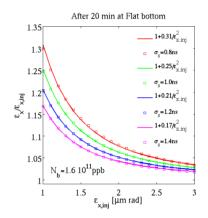
Figure 2: Parameterization of the IBS effect after 20 min at FB with the injected transverse emittance, for different input bunch lengths and for a bunch current of  $1.6 \times 10^{11} ppb$ .
