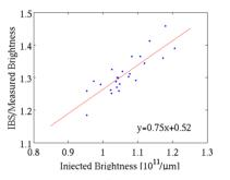
Figure 5: Parameterization of the unknown emittance blow up factor with the mean injected bunch brightness.
