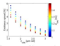
Figure 3: Parameterization of the emittance slope along the LHC train with the injected transverse emittance and bunch length.
