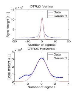
Figure 3: OTR2X vertical (top) and horizontal (bottom) beam profile images.
