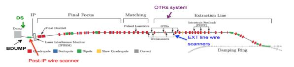
Figure 1: ATF2 beamline with the three different sections: EXT, FFS and the Post-IP line.
