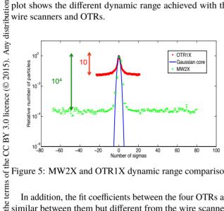
Figure 5: MW2X and OTR1X dynamic range comparison.
