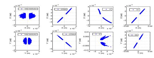
to the author(s), title of the work, publisher, and DOI. Figure 4: Gaussian beam halo model tracking through the ATF2 beam line. Phase space at: the beginning of the EXT line, OTR2X, IP and DS, note the difference on the scale, especially at the IP.
