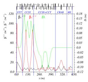
Figure 2: Optical functions of IR (version 6-14-3).
