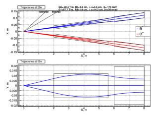
Figure 1: Trajectories of  $e^-$  and  $e^+$  bunches from IP through FF quadrupoles. Several lines are drawn at 10°, 15°, 20° to represent blind solid angle of the detector. Black rectangles over trajectories depict bare quadrupole apertures.
