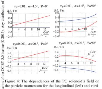
Figure 4: The dependences of the PC solenoid's field on the particle momentum for the longitudinal (left) and vertical (right) polarizations of the proton and deuteron beams.
