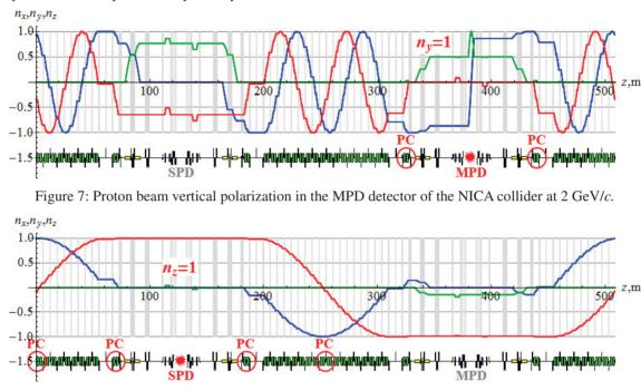
Figure 8: Deuteron beam longitudinal polarization in the SPD detector of the NICA collider at 13.5 GeV/c.
