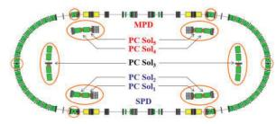
Figure 3: Placement of PC solenoids in NICA collider.
