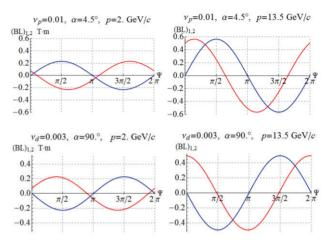
Figure 5: Dependences of the PC solenoid field integrals on the angle between the polarization and the beam direction  $\Psi$  for proton and deuteron mode of the collider.
