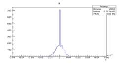
from this work may be used under the terms of the CC BY 3.0 licence ( Figure 9: The horizontal correctors' statistic after orbit correction.
