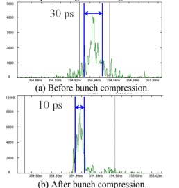
Figure 3: Bunch length measured by a streak camera before (a) and after (b) bunch compression at the chicane of injector section.
