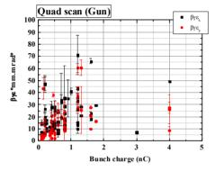
Figure 5: Emittance measurement results at the injector section by using the quadrupole scan method.
