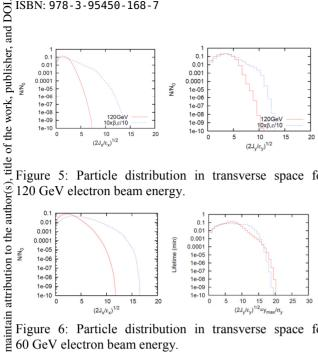
Figure 6: Particle distribution in transverse space for 60 GeV electron beam energy.
