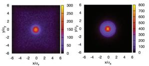
Figure 4: Electron distribution in the transverse plane during the interaction with a proton bunch in a drift space. The interaction times are z=-ct= $2.4 \sigma_z$  (left) and  $0.4 \sigma_z$  (right), where z=0 for the bunch centre.
