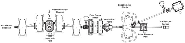
Figure 3: Schematic of interaction point as built.
