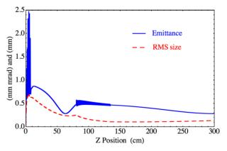
Figure 1: PARMELA beam dynamics simulation for a bunch charge of 100 pC.
