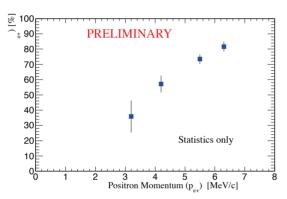
Figure 5: Preliminary results of the polarization of positrons produced in the PEPPo apparatus.
