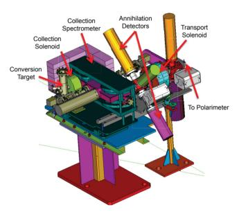
Figure 1: Vacuum beam line includes the insertable production target, a solenoid to collect e<sup>+</sup>, a double-bend spectrometer to define the momentum acceptance, a positron annihilation detector, and a second solenoid to transport e<sup>+</sup> to an exit vacuum window in front of the polarimeter.
