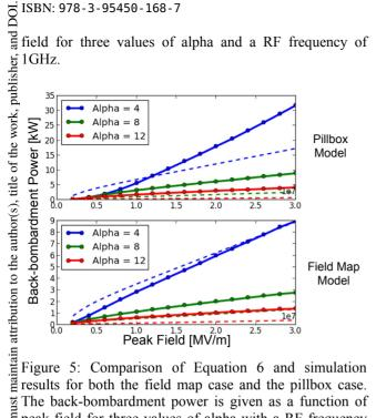
The back-bombardment power is given as a function of peak field for three values of class. of 1GHz.
