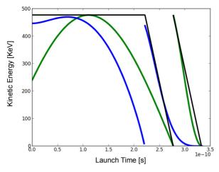
Figure 1: Comparison of numerical solutions to the equations of motion for a relativistic particle in a pillbox cavity (blue) with the approximation derived using Equation 5 for a particle traveling at a constant effective velocity (green) and linear model presented in the previous work (black).
