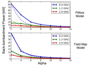
used under the terms of the CC BY 3.0 licence (© 2015). Any distribution of this work must maintain attribution to the author(s), title of Figure 3: Comparison of Equation 6 and simulation results for both the field map case and the pillbox case. The back-bombardment power is given as a function of alpha for three values of frequency with a peak field of 20MV/m.
