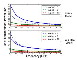
Figure 4: Comparison of Equation 6 and simulation results for both the field map case and the pillbox case. The back-bombardment power is given as a function of frequency for three values of alpha with a peak field of 20MV/m.
