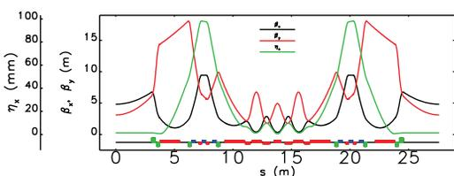
Figure 1: Twiss parameters in one sector of an alternate H7BA lattice design. Green blocks represent quadrupoles, red blocks represent dipoles, and blue blocks represent sextupoles.
