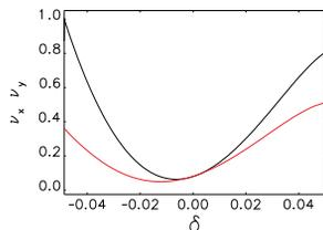
Figure 3: Horizontal (black curve) and vertical (red curve) betatron tune as a function of momentum offset  $\Delta E/E$ , dominated by second-order chromaticity.
