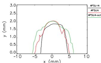
Figure 4: Dynamic acceptance (50<sup>th</sup> percentile) with physical apertures and errors, nominal lattice (black), alternate lattice with (green) and without octupoles (red).
