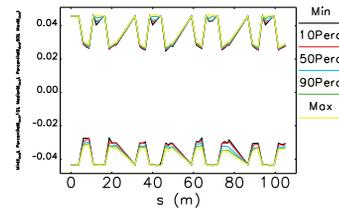
Figure 5: Local momentum acceptance with physical aperture and magnets errors, showing different percentiles.
