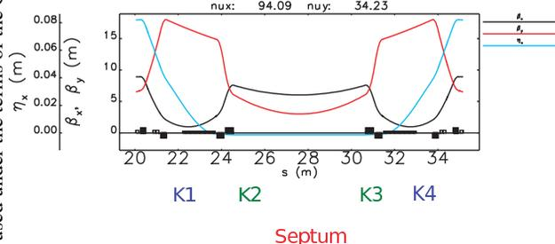
Figure 2: Layout of injection scheme with four injection kickers and a septum magnet.
