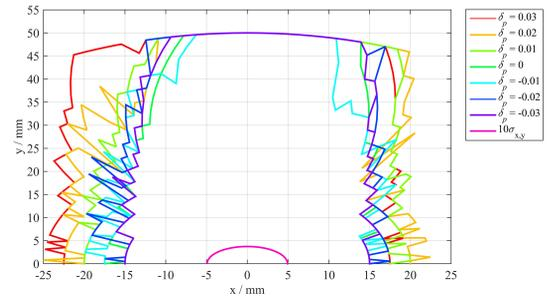
Figure 3: The dynamic aperture of the mini-beta lattice.
