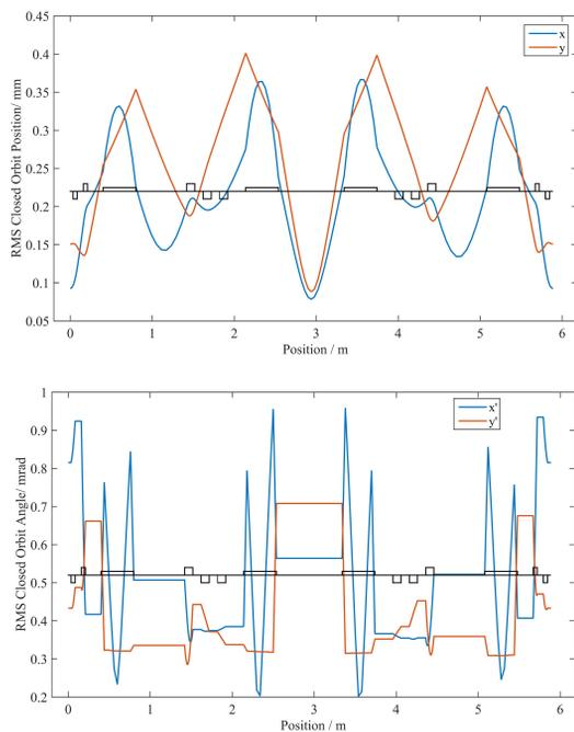
Figure 5: Uncorrected closed orbit.
