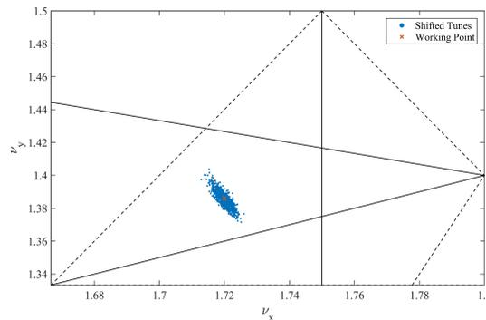
Figure 6: Tune spread due to field and misalignment errors.
