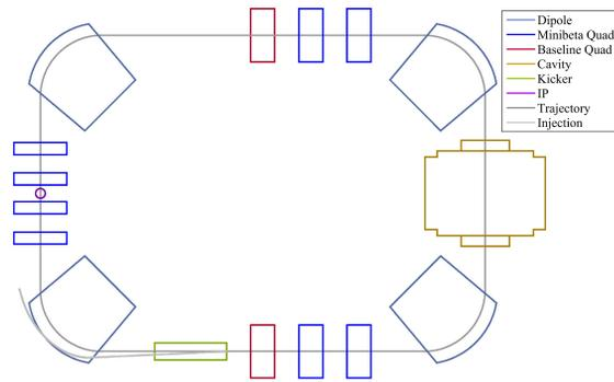
Figure 1: Layout of the mini-beta lattice.
