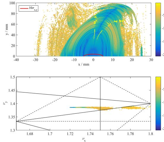
Figure 4: The dynamic aperture with diffusion rate of on-momentum particles.
