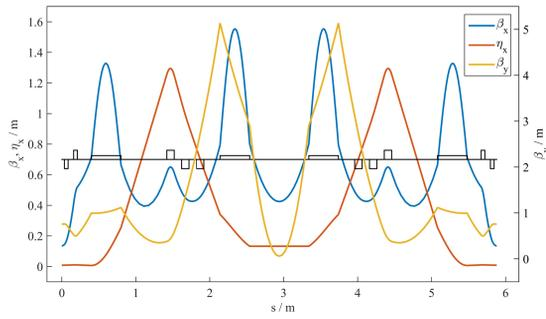
Figure 2: Optical functions of the mini-beta lattice.
