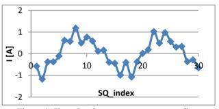
Figure 4: Skew Quads current to correct coupling.
