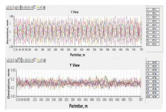
Figure 3: Residual vertical oscillations before (upper) and after (lower) correction with the same kicker excitation.
