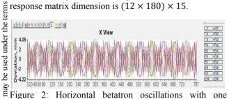
Figure 2: Horizontal betatron oscillations with one work horizontal kicker excitation.
