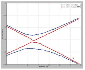
Figure 5: Tune separation measured before and after correcting linear coupling.
