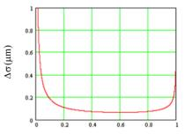
Figure 2: Error transfer from  $\Delta \gamma$  to  $\Delta \sigma$ assuming  $\Delta \gamma = 0.01$  as a function of  $\gamma$ .
