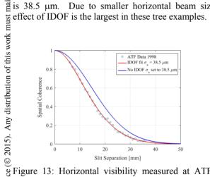
g Figure 13: Horizontal visibility measured at ATF as a g function of slit separation. Dots are measurements, red line is fitting Eq (4) and blue line is calculated visibility curve for a beam size 38.5µm *without* IDOF.
