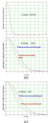
Figure 14: Calculated visibility curves as a function of double slit separation at the LHC. (a) beam size of 1.12 mm at 450 GeV. (b) beam size of 0.33 mm at 5 TeV and (c) beam size of 0.28 mm at 7 TeV
