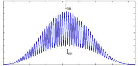
Figure 6: Typical interferogram at SPEAR 3. D=70 mm λ=550 nm.
