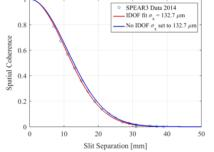
Figure 11: Horizontal beam visibility measurements at SPEAR3. Dots are measurements, red line is fitting Eq (4) and blue line is calculated visibility curve for a beam size  $132.7 \mu m$  without IDOF.
