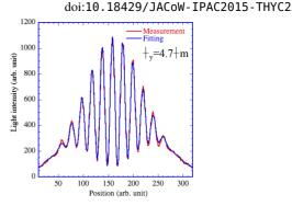
Figure 10: Interferogram at the KEK ATF. Red line is measurement, and blue line is fitting. Interferogram measured with D=60 mm and  $\lambda$ =400 nm.
