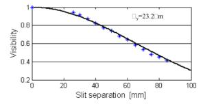
Figure 7: Visibility as a function of double slit separation at SPEAR3. The dotted line is measurement result, and the solid line is a Gaussian fit.
