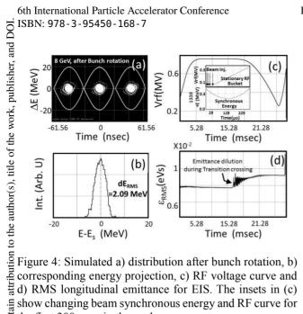
show changing beam synchronous energy and RF curve for the first 300 μsec in the cycle.
