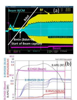
Figure 5: A measurement data on early injection scheme: a) Scope data for the first 1 ms after beam injection (pink trace is -1×Beam) b) 13BT beam, total RF voltage and loss monitor data from injection to extraction without notch in the beam. The beam efficiency was nearly 94% in this case.
