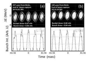
Figure 2: Simulated phase space distributions (top) and time projection (bottom) just before beam acceleration for a) CIS and b) EIS.
