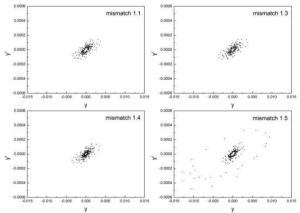
Figure 4: The position of beam-core particles in phase space with different mismatch factor.
