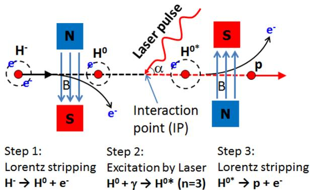
Figure 1: Schematic view of laser-assisted  $H^-$  stripping.
