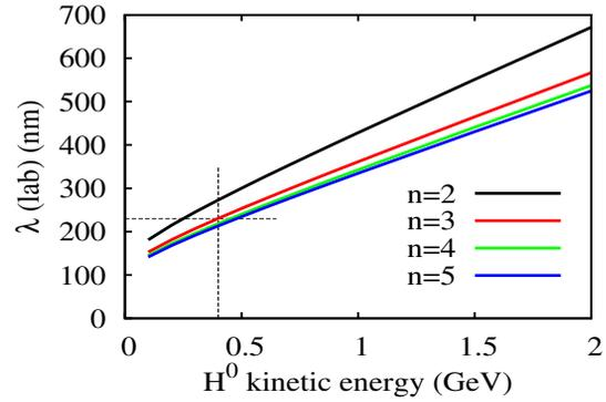
Figure 3: Doppler shift of the transition wavelength of  $H^0$  as a function of its kinetic energy is calculated by using Eqn. 1.  $n$  is the principal quantum number of hydrogen atom. Laser wavelength for 400 MeV is required to be 230 nm.
