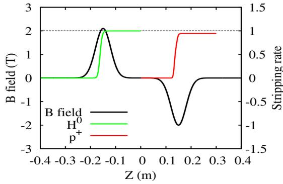
Figure 2: Magnetic field configuration and Lorentz stripping rate of  $H^-$  and  $H^0$ \*
