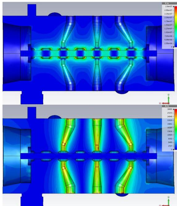
Figure 4: Electric (top) and magnetic (bottom) fields.
