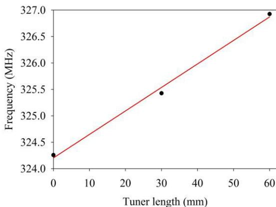
Figure 7: Tuner frequency shift vs the tuner position synchronous motion of all four plungers.
