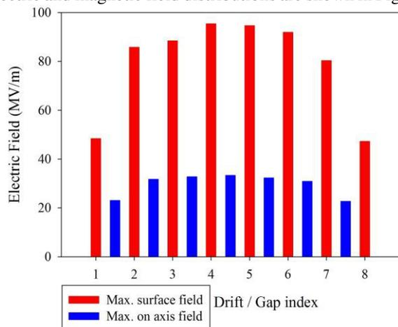
Figure 3: Maximum drift tube surface fields versus the maximum on axis gap fields.
