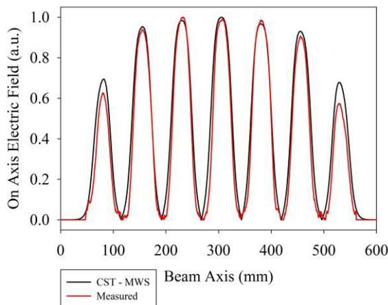
Figure 5: The measured on axis field compared with the simulated one by CST.
