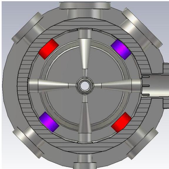
Figure 6: Magnetically acting tuner positions (in red at the cavity entrance, in magenta at the cavity end).
