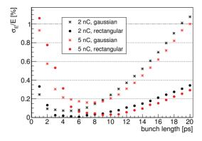
Figure 7: Energy spread at the end of 5-sector as a function of the bunch length with optimal RF phase.
