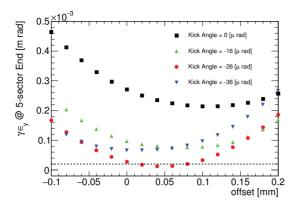
Figure 5: Vertical emittance as a function of offset and kick angle when the beam charge is 5 nC.
