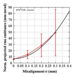
Figure 2: Vertical emittance at the end of 5-sector as a function of the magnitude of misalignment.
