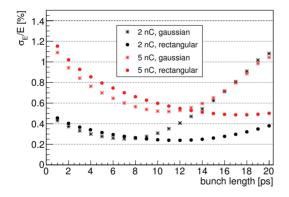
Figure 6: Energy spread at the end of 5-sector as a function of the bunch length with on-crest RF phase.
