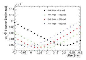
Figure 4: Vertical emittance as a function of offset and kick angle when the beam charge is 2 nC.
