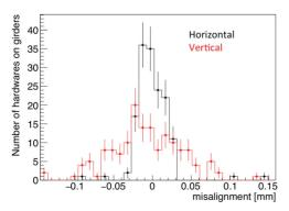
Figure 3: Measured misalignment of the accelerator structures on the girders in the horizontal (black) and vertical (red) direction.
