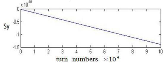
Figure 4: EDM signal growth vs. turn number.
