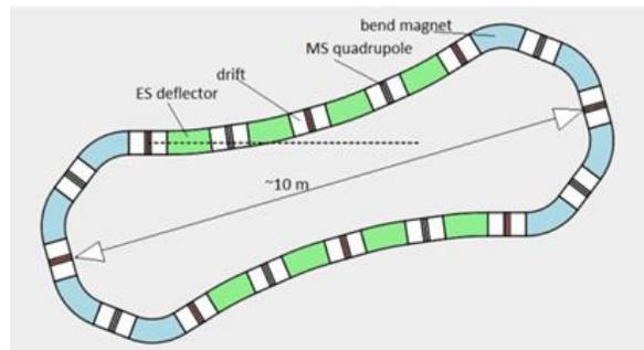
Figure 2: Ring lattice based on QFS concept.
