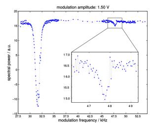
Figure 5: Spectral power at the synchrotron frequency  $f_s = 16.05$  kHz of all bunches for variable modulation frequencies. Coupled-bunch instability suppression is maximized for  $f_{\text{mod}} = 31.6$  kHz and also achievable for  $f_{\text{mod}} = 47.8$  kHz.
