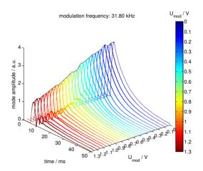
Figure 3: Grow-damp measurements for different amplitudes of the RF phase modulation with a modulation frequency of  $f_{\text{mod}} \approx 2 \cdot f_{\text{s}} = 31.8$  kHz. Exponential fits to determine the damping rate are not viable for amplitudes above  $U_{\text{mod}} = 0.5$  V.
