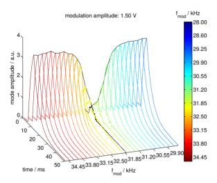
Figure 4: Grow-damp measurements for variable modulation frequencies  $f_{mod}$  with the synchrotron frequency  $f_s = 16.05$  kHz. The suppression of multibunch mode 12 is maximized for  $f_{mod} = 31.8$  kHz (black curve).
