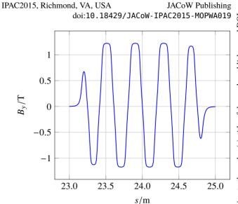
Figure 3: Vertical field  $B_y$  as a function of the longitudinal position on the beam axis.
