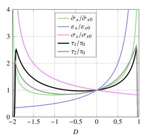
Figure 2: Average bunch width around the ring  $\bar{\sigma}_x$ , hor. emittance  $\varepsilon_x$ , bunch length  $\sigma_s$  and lifetime  $\tau_{1/2}$  as a function of damping partition D, divided by corresponding D = 0values. Lifetime calculated for:  $\tau_1$ : constant vertical beam size  $\sigma_{v}(D) = \text{const.}; \tau_{2}$ : for constant emittance coupling  $\sigma_{v}(D) \neq \text{const.}$
