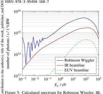
Figure 5: Calculated spectrum for Robinson Wiggler, IRdipole and EUV-dipole at the MLS with the existing apertures and a beam current of 200 mA.
