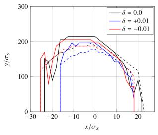
Content from this Figure 6: Dynamic aperture for the MLS without Robinson Wiggler calculated with MAD-X (dashed) and the self-written code (solid) for different energy deviations.  $\sigma_x = 966 \,\mu\text{m}, \, \sigma_y = 42 \,\mu\text{m}, \, \eta_x = 0.17 \,\text{m}$
