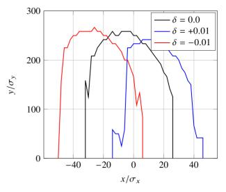
Figure 7: Dynamic aperture for the MLS with Robinson Wiggler calculated for different energy deviations.  $\sigma_x = 701 \,\mu\text{m}, \sigma_v = 36 \,\mu\text{m}, \eta_x = 0.54 \,\text{m}$
