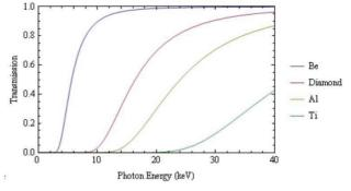
Figure 2: Transmission energy dependence for several windows.
