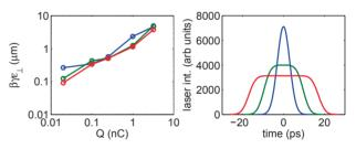
Figure 3: Left: simulations of transverse normalized emittance at ASTA for different bunch charges. Simulations were performed with different laser longitudinal profiles (right).
