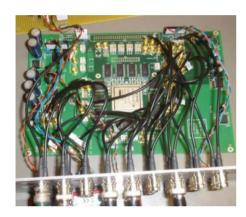
Figure 3: FONT5 digital feedback board.
