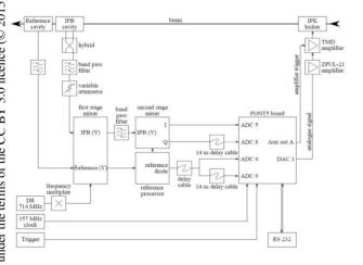
be used Figure 4: Schematic of configuration of IP feedback system.
