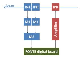
Figure 2: Schematic of IP feedback system showing the cavity BPM (IPB), reference cavity (Ref), first and second down-mixer stages (M1 and M2), FONT5 digital board, amplifier and kicker (IPK).
