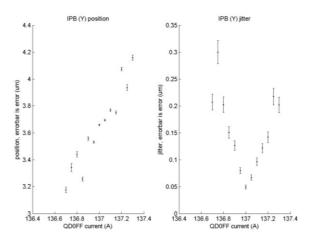
Figure 8: Bunch two mean position (a, left) and position jitter (b, right) vs. QD0FF current.
