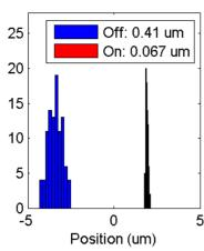
Figure 5: Distribution of the vertical position of bunch two in IPB with (red) and without (blue) application of the IP feedback correction.
