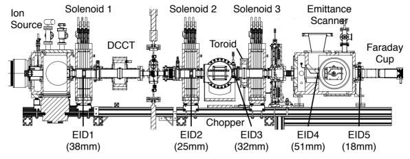
Figure 1: A schematic of the PXIE LEBT beam line, highlighting the beam diagnostic devices.
