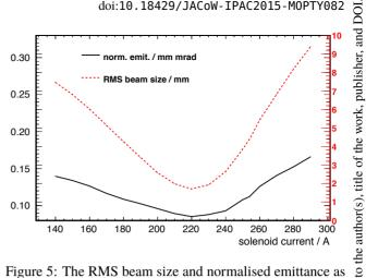
Figure 5: The RMS beam size and normalised emittance as seen at the Allison scanner as a function of solenoid three current.
