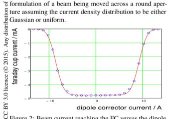
Figure 2: Beam current reaching the FC versus the dipole corrector current. Blue circles are measurements, and the solid red curve is the fit which produces a value for beam size and beam centre.
