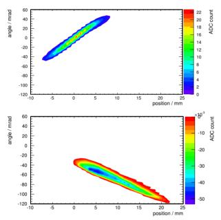
Figure 4: The phase space as recorded by the Allison scanner, for a 5 mA H<sup>-</sup> beam (top), and the associated positive signal (bottom). Note the change in intensity scale for each plot.
