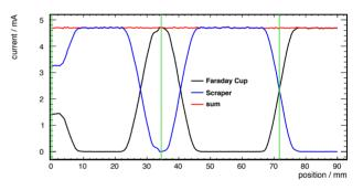
Figure 3: Currents (inverted) of the LEBT scraper and Faraday Cup as functions of the LEBT scraper position. The vertical green lines represent the positions of the 5 mm, 14 mm, and straight edge openings respectively.
