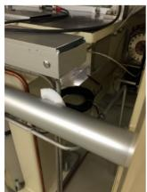
Figure 5: When the sponge obstructs the water pipe vibration, the PSD stability is improved immediately.
