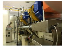
Figure 2: Laser potion and isolation tube of Laser -PSD system are assembled on the side of girder in lab. Then magnet girders are transported back and placed on pedestals in TPS tunnel.
