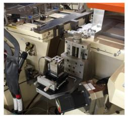
Figure 8: The reference laser is set on pedestal for recalibration.
