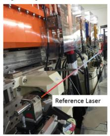
Figure 9: The reference PSD will be installed on girder for adjusting the reference laser to parallel to the datum plane of front girder.
