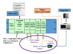
Figure 2: EPICS IOC layout for TPS pulse magnet power supply control.
