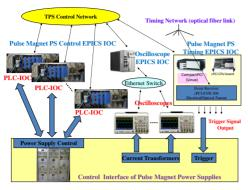
Figure 1: Control environment of TPS pulse magnets power supplies.
