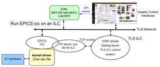
Figure 1: System architecture of EPICS IOC on TLS ILC.
