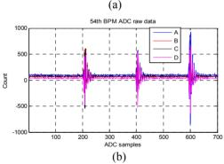
Figure 3: (a) The ADC data when beam passes through the 1<sup>st</sup> BPM of the booster synchrotron on the first day of Booster commissioning. (b) The ADC data as the beam had stored in the booster.
