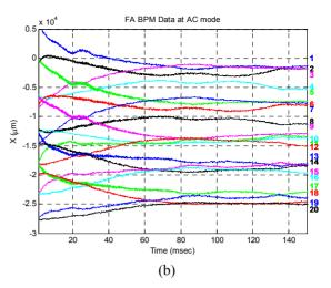
Figure 8: (a) DC mode Orbit. 60 Hz orbit perturbation is mainly from quadrupole power supply ripple. Horizontal Phase advance around adjacent BPMs is around  $\pi/4$ . Resolution of BPM is gradually deteriorated after 120 msec due to beam loss. (b) AC mode Orbit. Close orbit variation during ramping could be over 6 mm before tune and orbit correction and then reduced between 3 mm after tune correction.
