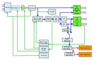
Figure 2: BPM platform functional block diagram.
