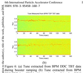
during booster ramping (b) Tune extracted from BPM TDP TBT data. TDP had better signal qualities than DDC due to its clear and no smear TBT data.
